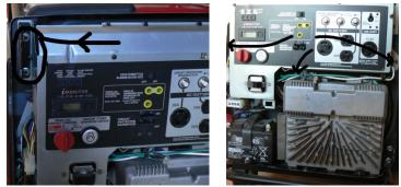
5. Carefully tip down the control panel to access the rear.
