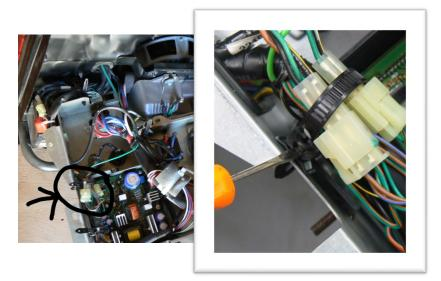
7. Unplug both the ignition switch and start switch connectors. Rotate the plastic tie 180 degrees to ease reattaching it later.
