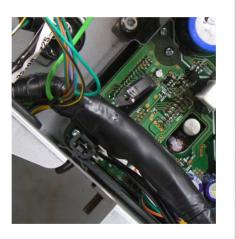
8. Connect the GenStart Module to the Ignition and Start Switches. Position the module and connect to generator as shown, route battery wiring towards battery.
