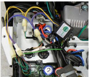
9. Position the module, wiring and all connectors as shown. Use plastic tie to secure Module to generator harness and reattach tie from step 6.
