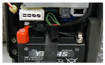
11. Pass the 6" Control Harness through the battery cover as shown. Connect to GenStart Module and reinstall cover.
