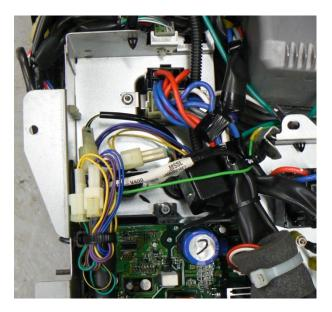
10. Reassemble generator in reverse order of disassembly. Pass Start System red battery terminal through back side of generator positive battery protective boot and connect both Start System red terminal and generator positive terminal to battery. Connect Start System black battery terminal and generator negative terminal to battery. Route wiring as shown.
