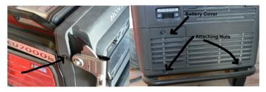
4. Carefully remove foam insulation from around the handle bar brackets. Using a 12mm socket, remove 4 attaching bolts. Remove brackets. Using a 10mm socket remove 3 remaining nuts on control panel, note the nut on the left has a protective plastic cap that must be re-installed.
