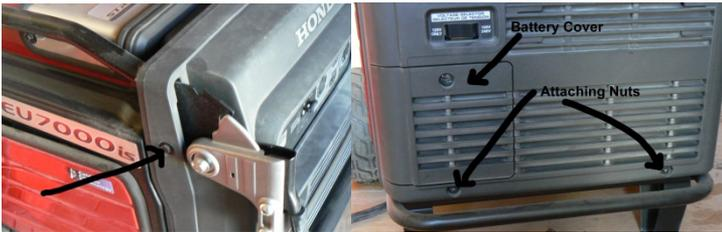
4. Carefully remove foam insulation from around the handle bar brackets. Using a 12mm socket, remove 4 attaching bolts. Remove brackets. Using a 10mm socket remove 3 remaining nuts on control panel, note the nut on the left has a protective plastic cap that must be re-installed.
