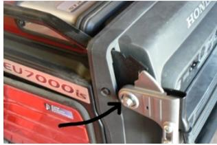
3. Using a 10mm socket, remove 2 bolts and 2 nuts attaching front cover. Carefully remove front cover making sure you do not lose the metal bushings on the lower studs.
