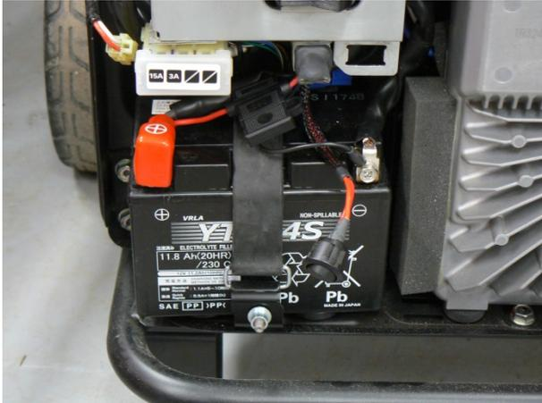
13. Re-install generator front cover. Do not install battery cover at this time.
