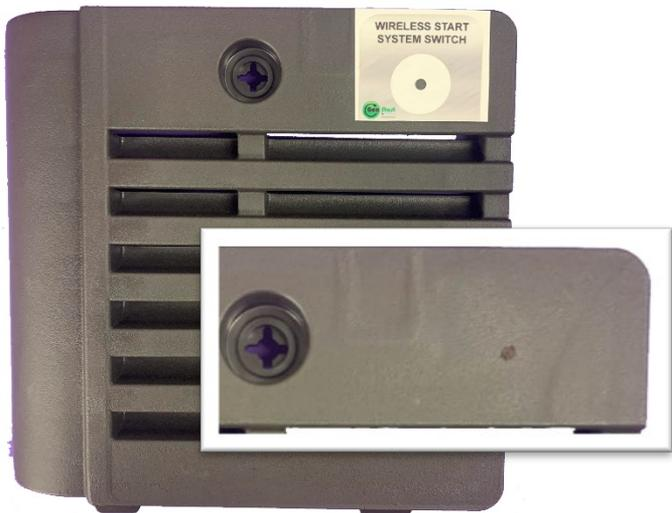
15. Drill a 1/8 pilot hole through the cover on the center mark made in step 12. Enlarge the pilot hole to 3/4 inch using a hole saw or step drill. Carefully file a small notch on the left side of the hole to receive the index tab on the back of the supplied panel switch. Test fit the panel switch frequently.
