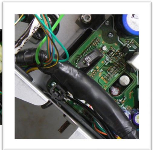
8. Connect the GenStart Premium Start Module to the Ignition and Start Switches as shown.
