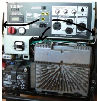
5. Carefully tip down the control panel to access the rear.
