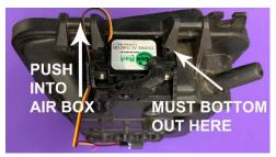
16. Carefully pull down on choke actuator wire till snug.
