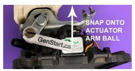
18. Reattach choke cable making sure the choke cable spring goes in the recessed side of the carburetor choke lever.
