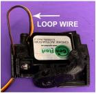
15. Install choke actuator as shown. Place the actuator on top of the air cleaner and push into place until fully seated.
