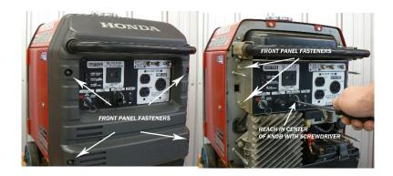
4. Locate precut hole in center rear of control panel. Using drill with step drill bit, drill a small hole through the control panel faceplate to mark hole location. From the front of the panel enlarge hole to 20mm (3/4-inch). Be very careful not to damage any wiring with drill bit.
