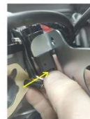
1e-4/5 Remove cable harness support bracket by first removing black plastic push in connector. Use pliers to press backside of small push through and pull from other side to release. Then press tab on larger connector and pull down and away. Save gasket after removing from silver plate.
