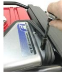
1a-2/3 Pull back rubber gasket and remove 2 #10mm nuts then pull up and remove corner cover.
