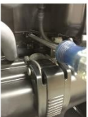
1e-1/2/3 Remove final piece of airbox from throttle body by removing inner two #10mm nuts, loosening clamp below and then swinging plastic box off studs and pulling up.
