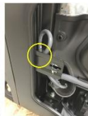
1d-1/2 Gently twist tank vent tube and insert into forward hole on backside of door latch for safe keeping.
