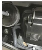
1d-3/4 Pull up canister vent tube from white plastic clip and pull out of hole to make room for adding new vent line.
