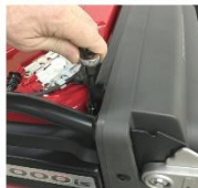
1c-2/3 Locate and remove four #10mm corner bolts with washers as final step before lifting out tank.
