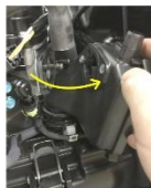
1e-1/2/3 Remove final piece of airbox from throttle body by removing inner two #10mm nuts, loosening clamp below and then swinging plastic box off studs and pulling up.
