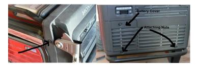
4. Peel back self adhesive strip from Velcro on the back of the 2-Wire Start Module and attach it to the generator as shown. Be sure the module is low enough that the battery connections will reach the battery. Connect the remote control wiring connector on the 2-Wire Stat Module to the generator remote start connector.
