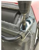
2e-3/4/5 Re-install exhaust shield with 4 10mm bolts then install 2 handles with qty 4 each 12mm bolts.
