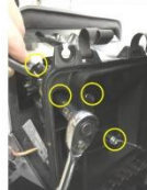
2b-4 Tighten 2 removed 10mm nuts and new 10mm bolt placing 4 supplied washers between frame and air box.
