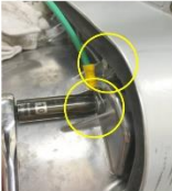
2c-2 Secure ground strap from gas module to either frame bolt.
