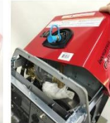
2c-4/5/6 Reposition top gasket so facing forward, then re-install pull handle assembly then pull up on gas module and tilt front edge of lid down to install cover over gas module.
