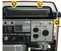
2d-3 Re-install front 3 cover 10mm bolts
