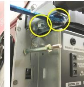
2e-3/4/5 Re-install exhaust shield with 4 10mm bolts then install 2 handles with qty 4 each 12mm bolts.
