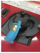
2e-1/2 Install supplied 2 clamp halves on top of unit then tighten 2 clamp bottom 5/32" socket head bolts on underside. USE CAUTION- BEWARE OF SHARP EDGES ON SHEET METAL FRAME.
