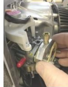
2b-2/3 Install gasket from removed choke assembly then install supplied injector assembly followed by supplied gasket (or optionally supplied liquid gasket to be applied from tube)
