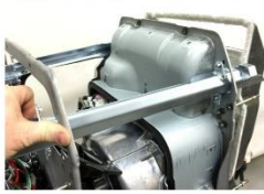
2a-1 Re-install side rail, loosely install 8 removed 10mm bolts then tighten all bolts to secure frame.
