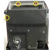
2d-4/5 Re-install rear 3 cover 10mm bolts where 2 are partially hidden under exhaust baffle top edge.
