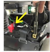
2e-6 Connect & tighten battery terminals connecting red lead first then black lead.
