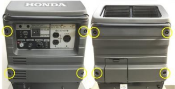
2f-1/2 Re-install front and back covers with 4 each 10mm cap nuts
