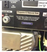
2a-2 Install supplied label over holes or eye bolt and plug (if supplied) into front box then re-install box with 4 removed 10mm bolts.
