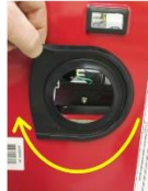
2c-4/5/6 Reposition top gasket so facing forward, then re-install pull handle assembly then pull up on gas module and tilt front edge of lid down to install cover over gas module.
