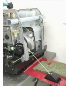
2c-4/5/6 Reposition top gasket so facing forward, then re-install pull handle assembly then pull up on gas module and tilt front edge of lid down to install cover over gas module.
