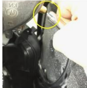
2c-3 Install vent tube on regulator so bottom end goes down into base rail and top into gas regulator brass nipple.
