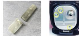
2f-1/2 Place large end of catalyst insert into spark arrestor then insert spark arrestor back into muffler inlet. Re-attach muffler to engine with qty 3 10mm bolts where the longer bolt installed at the lowest hole.
