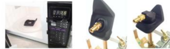
2a-2/3/4 Remove Honda gas boot from old gas tank and install over inlet (heat with hot water or carefully microwave for 15 seconds to soften it) CAUTION - RUBBER WILL BE HOT WEAR SUITABLE GLOVES.
