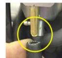
2h-4 If a high-altitude kit is used change the fuel jet in the end of the fuel tube with the supplied allen head wrench.
