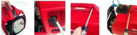
2g-1/2/3/4-install side skins by first installing "wood" screw above pull starter then install top two screws starting with back end screw.
