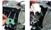
2c-3/4 Re-install gasket then slide carburetor back on. Make sure servo wire is not tight on left side.
