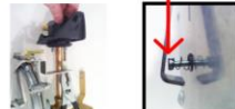
2a-5/6/5 Re-install air purge knob & shaft then adjust for 1/8" (+/- 1/16") clearance between spring button and lever. DANGER - MAKE SURE THERE IS A GAP or you will have propane leaking when you connect to your BBQ tank!
